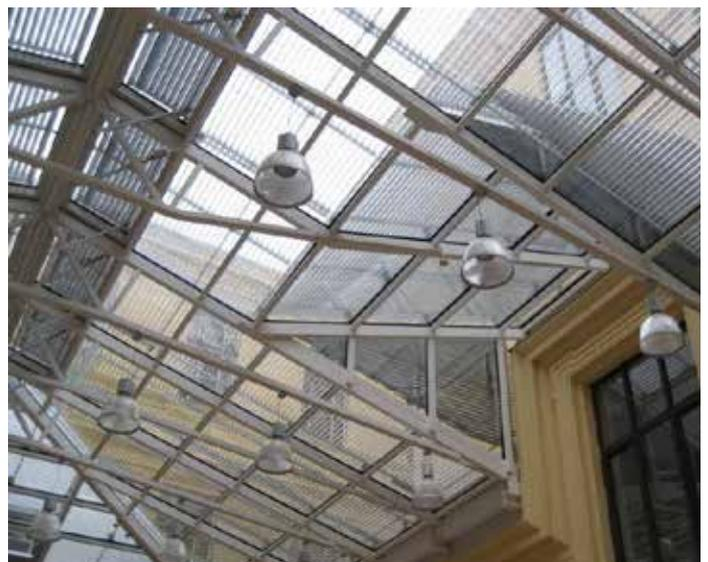
Horiso Rack Arm Systems can also be installed internally, providing additional benefits to an interior space. Heat gain, glare and airflow can be controlled throughout the day. Interior Rack Arm Systems are perfect interior shading options for sloped glazing, skylights, angular, shaped and high glass windows.
